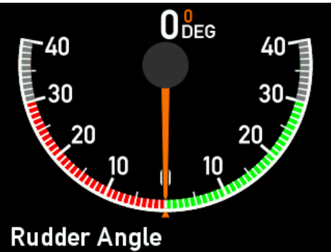
Example of XDi 96 D scale configured to \pm 30^\circ .
